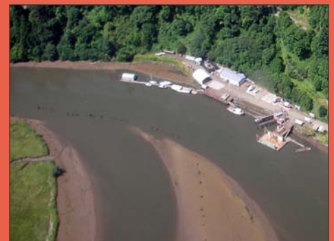
The current channel depth has several areas at -10 so larger vessels schedule arrival and departure times with the tides.
